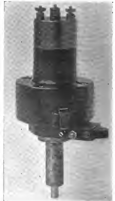
Pittsfield ignition unit. The cam C first lifts blade A so closing the contacts, and then raises the fiber block F so lifting blade S and positively separating the contacts again. P is a wick for supplying oil to the cam
